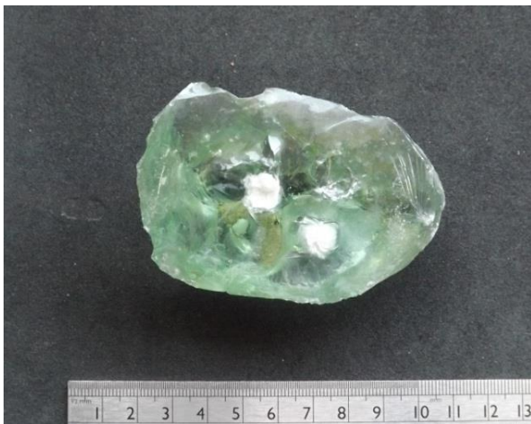
Glass waste, showing quartz inclusions, from the kin site
